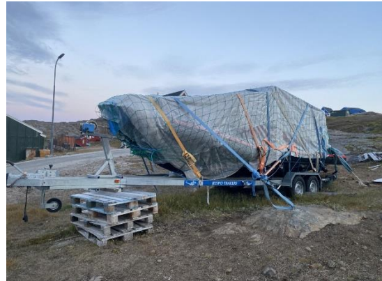
New winter cover for “Rana”; note the ground tie-downs.
