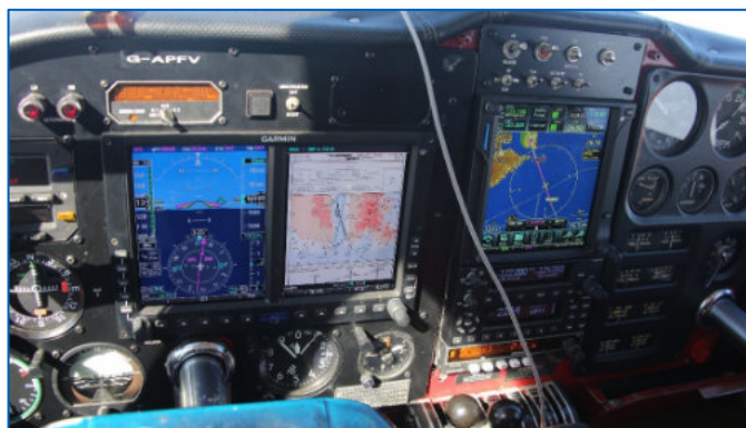
Digital cockpit in a 1958 vintage aircraft, complete with autopilot and satellite telephone. Mid-way between Egilsstadir (BIEG) and Constable Pynt. Altitude: 10,000 ft, ground speed 143 mph. Approach plate for Constable Pynt on the display
